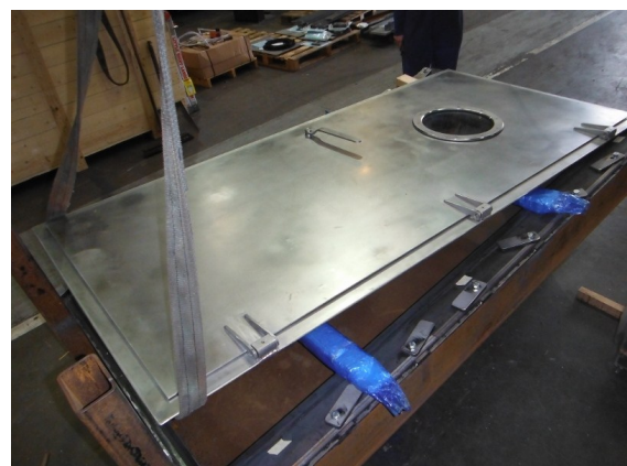
The gastight doors were tested using Westmoor's in-house test facilities
