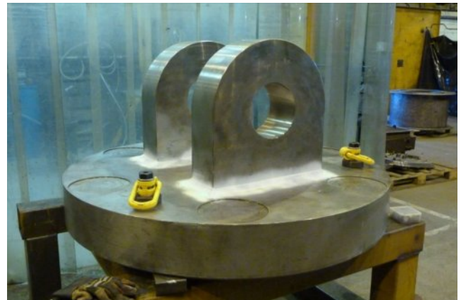
Padeyes welded into the base plate
