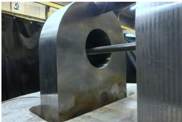
Padeyes positioned into re-machined slots ready for welding
